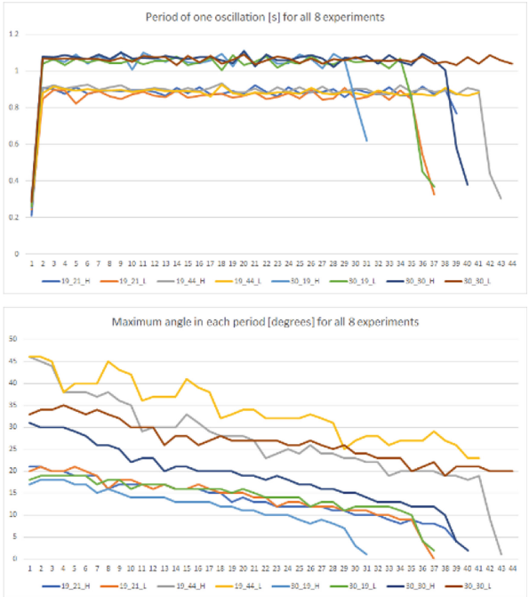
Fig. 14. Visualization of the oscillations: period depends only on the pendulum length (top) and remains constant while the pendulum moves; max amplitude decreases over time (bottom).
