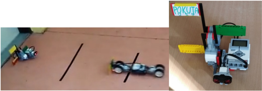
Fig. 1. Measuring speed with ultrasonic sensor, from Robot League 8/2018, team Šachisti.
