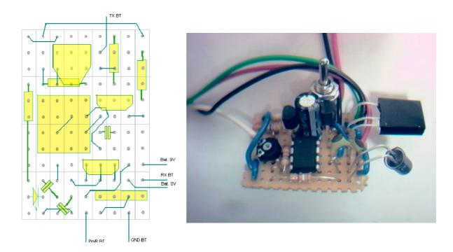
Figure 4. Serial to IR bi-directional converter. The board on the left is from the point of view of the parts. The switch is installed between the two pads, where the 9V battery cable connects. This design utilizes two parallel 47pF capacitors instead of the single 100pF shown on the schematic above.
