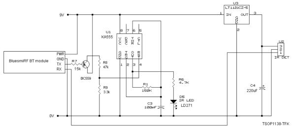
Figure 2. Schematic for the bidirectional IR to serial converter. Designed in cooperation with Ing. Richard Balogh, Faculty of Electrical Engineering, Slovak Technical University, Bratislava. The value of R1 should be tuned with the oscilloscope so that the frequency on pin 3 of U1 will be 38kHz (our value is 128kOhm). In our realization, we replaced the low dropout voltage regulator LT1121CZ-5 with an equivalent LM2931AZ-5.0. According to the documentation, C4 needs to be at least 100uF.
