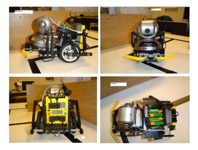
Figure 1. Robot built by Jean Paul Franky Friquin as part of his diploma project. The image is transmitted to the PC workstation, and the victims are detected. In case a victim is found a signal is sent to the RCX to stop, beep, and signalize the presence of the victim.
