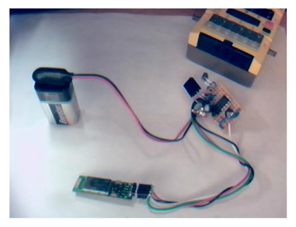
Figure 5. The device is powered from 9V battery. The BlueSmiRF module can be unplugged and used in other designs when needed. It can also be places comfortably at a separate location - such as on top of the robot for best RF transmission.
