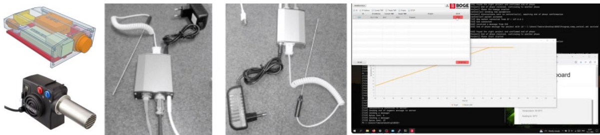
Figure 3. Software (and hardware) for controlling industrial hot-air burner shown on bottom the left.
