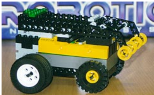
Figure 2. Simple robot with a front bumper used at the first lesson.
