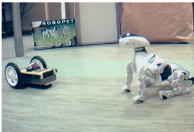
Figure 2. Controlling RoboPet from RCX using IR signals.
