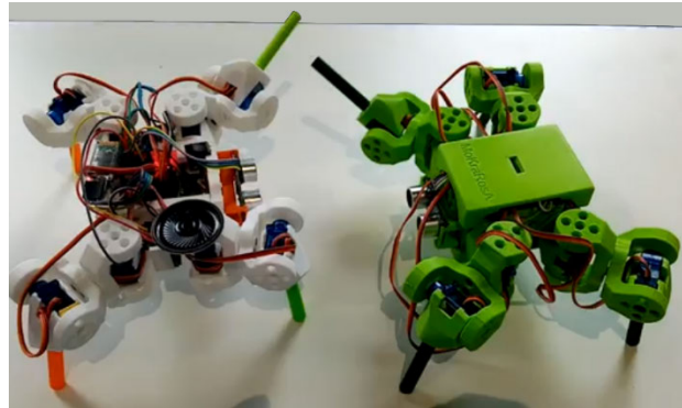
Figure 6. MoKraRosA, version 1 (left) and version 2 (right). Version 2 has been designed after the summer camps and provides a “shelf” for every electronics part included.
