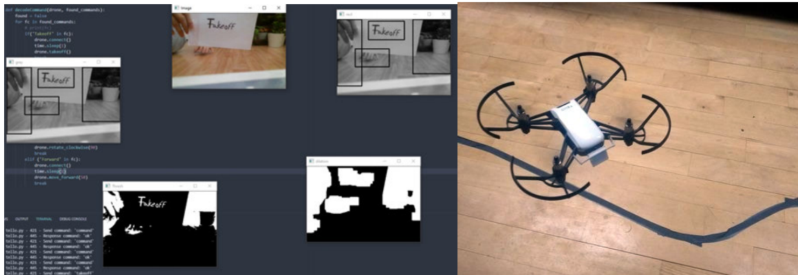
Figure 9. Controlling drone with signs using optical character recognition (left), line-following robot (right).
